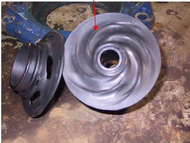
Figure 3 – Front of impeller, no vanes
