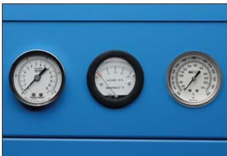
*Inlet filter differential, blower exhaust temperature and pressure gauges are standard.*
