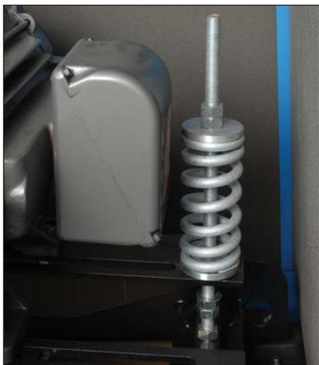
*Roots patented automatic V-belt drive tensioning system.*
